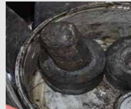
Lead source pin for density gauge (Cs-137) 20 July 2009
