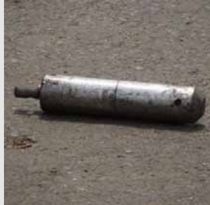
Damaged soil density gauge rod (Cs-137) 4 October 2010
