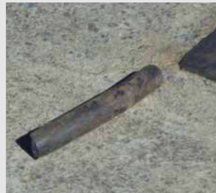
Radiation source (Cs-137) Troxler shaft 1 August 2016
