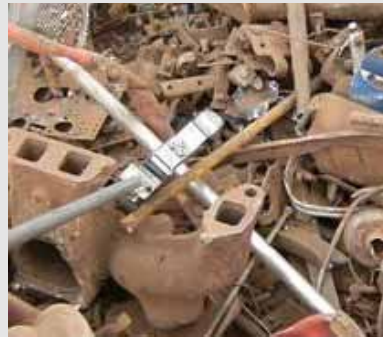
Damaged soil gauge rod (Cs-137) 14 May 2011
