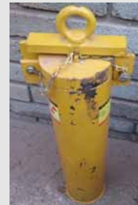
Custom made container with Troxler soil gauge rod (Cs-137) 25 Sept 2014.
