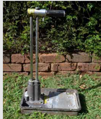
Damaged Troxler soil density gauge (Cs-137) 3 December 2014
