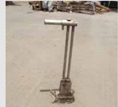
Damaged soil density gauge (Cs-137) 3 November 2010
