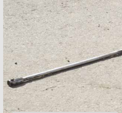
Damaged soil gauge rod (Cs-137) 14 October 2010
