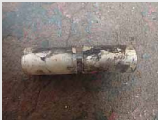
Radioactive fuse (Ra-226) 2 September 2020
