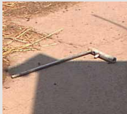
Damaged soil density gauge (Cs-137) 30 March 2004
