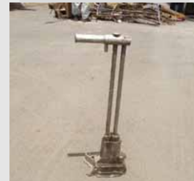
Damaged soil density gauge (Cs-137) 3 November 2010
