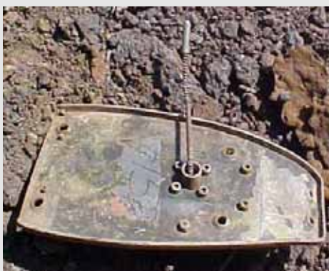
Damaged radiography camera with 'pigtail' (Iridium-192) 1 December 2003
