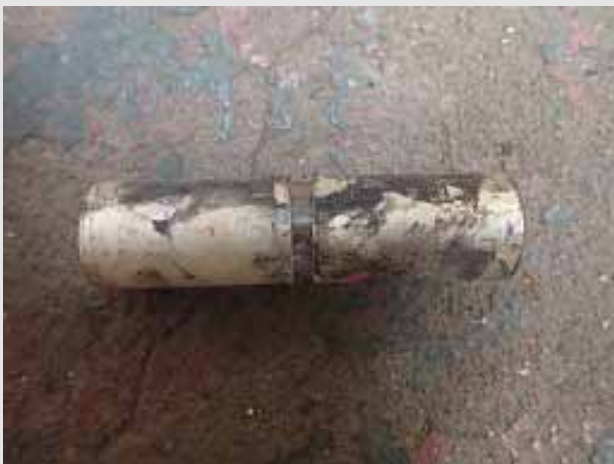
Radioactive fuse (Ra-226) 2 September 2020
