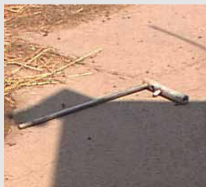
Damaged soil density gauge (Cs-137) 30 March 2004
