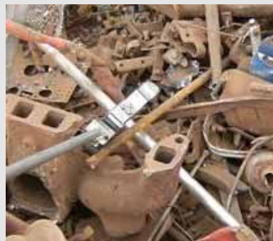
Damaged soil gauge rod (Cs-137) 14 May 2011
