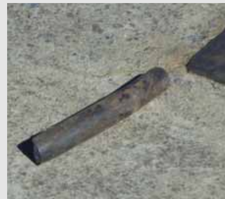
Radiation source (Cs-137) Troxler shaft 1 August 2016
