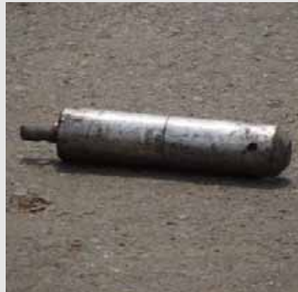
Damaged soil density gauge rod (Cs-137) 4 October 2010
